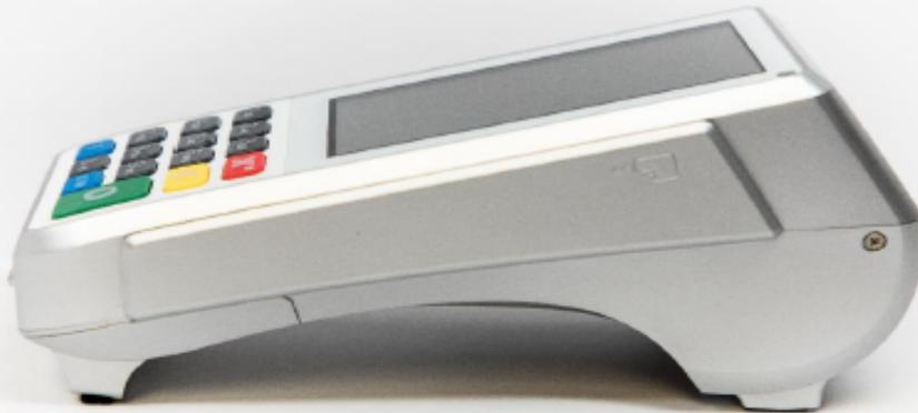
The MSR slot is located on the right side of the device. Please inspect it to make sure that no foreign devices are attached or inserted, and ensure that the area is free of any obvious tamper marks such as tool marks.
