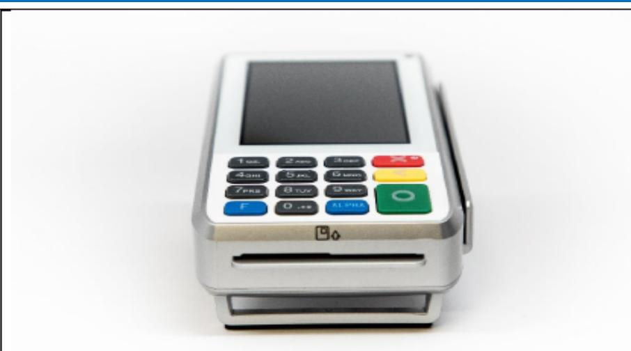
The EMV slot is located on the front end of the device. Please inspect it to make sure that no foreign devices are attached or inserted, and ensure that the area is free of any obvious tamper marks such as tool marks.
